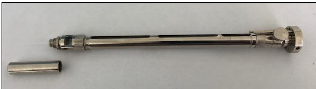
Figure 7. High-capacity Harbo syringe (original).
