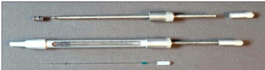
Figure 6. Schley syringe (source: http://www.besamungsgeraet.de/_en/insemination-instruments/ ).
