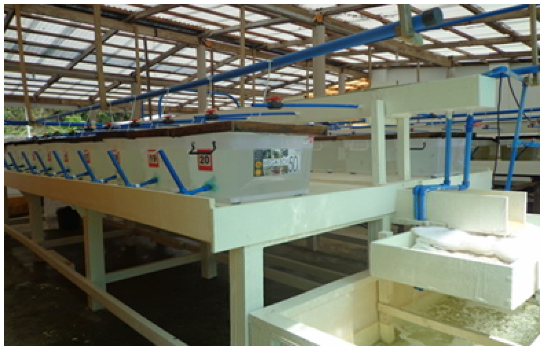
Figure 1. Recirculating system used in the feeding trial made up of twenty 50 L aquaria and biological and mechanical filtration.
